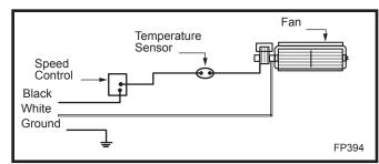
Fig. 8 Wiring diagram.
